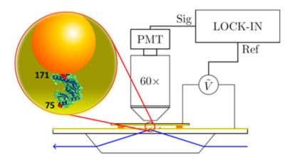
The figure shows schematically a nano-rheology setup which allows sub-Angstrom resolution measurements of enzyme deformations.
